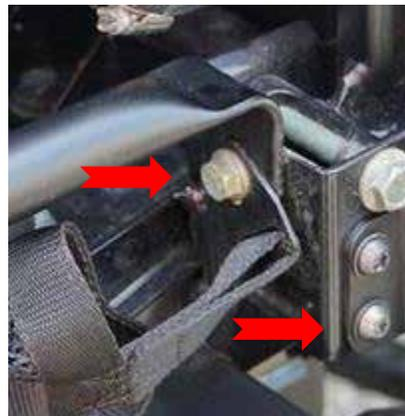
12) Remove net and reinstall bolster bar using 8mm bolt previously removed.
