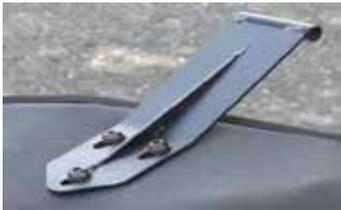
20) At handle locations shown, mark area on fabric for (3) 6mm bolt to go through. Using #2 Philips head screwdriver punch holes through the fabric at previously marked location.
