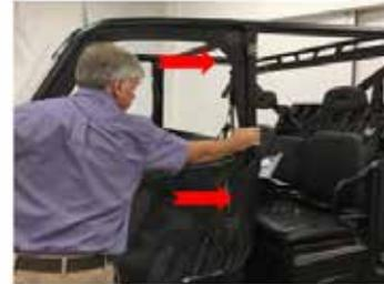
32) Close door and whole holding front of door tight to ROPS, tighten (2) 6mm rotary latch bolts.
