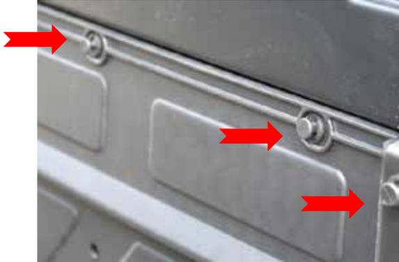
7) Remove 2 lower T40 torx screws and set set aside to reuse.
