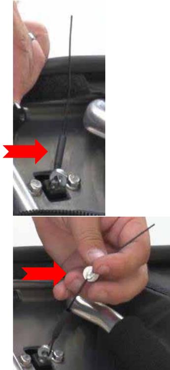
25) Insert bolt with cable up through rotary latch. Install 6mm locknut. Adjust cable so it has about 1/4" slack and tighten locknut. Insert open end of cable through shrink tube. Heat shrink with heat gun or lighter.
