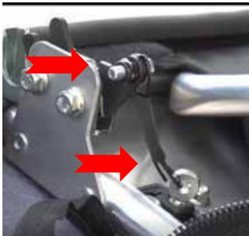
26) Loop door limiter strap around frame tube and back through loop on limiter strap. Insert end of limiter strap through slot on inner side of door skin.
