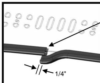
Co-extruded bulb seal starting/finishing point
