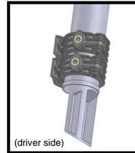
To apply more or less tension to the roll cage, simply rotate the clamp handle from the tension screw as shown below. Over tightening clamps to roll-cage could cause parts failures.
