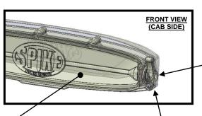
As shown on the front-view image, the <u>lever</u> is installed by default on the right side of the vent.
