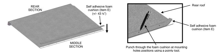
d) Assemble the front and the rear roof together using supplied hardware (Item F) as shown below.
