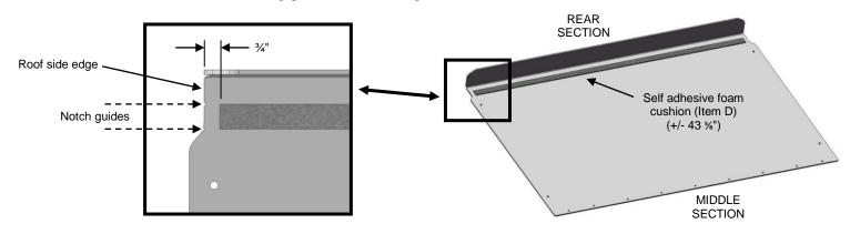
c) Apply the self-adhesive foam cushion (Item E) to the front side of the rear roof (Item B) as shown. For proper installation, the roof must be free of any dust or any other contamination. Using a pen, screwdriver or any other similar pointy tool, pierce through the foam cushion using the rear roof mounting holes as guides (9 locations).
