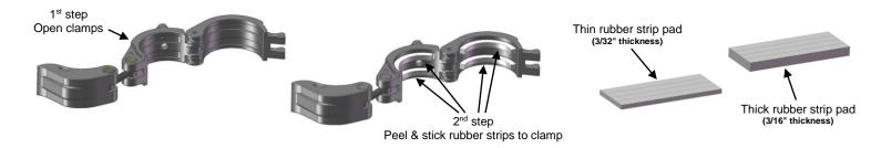
h) Attach the clamps to the roll-cage as shown below and pre-adjust tightening tension of all clamps. NOTE: Keep all clamp handles open as shown in step 3 below; this will allow you to move the clamps left or right when installing the roof for the first time.
