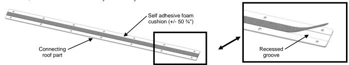
b) Find a clean flat area where you can safely lay down the front roof part (Item A) and partially remove protective film from the back side. Precut 2 strips (2 x 21") of the self-adhesive foam cushion (Item F) and apply them to the front roof part as shown below using manual pressure to ensure good adhesion. For proper installation, the roof must be free of any dust or any other contamination.
