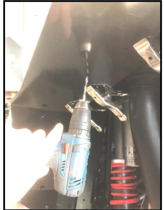
**WARNING: For each guide mounting hole, a single (1) layer of OEM front left lateral panel should be drilled / pierced**
