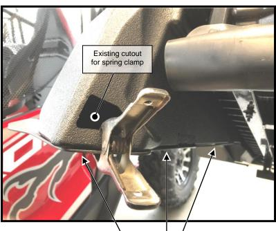
Ensure that fender flare edges line-up with the inside edges of the dump bed
