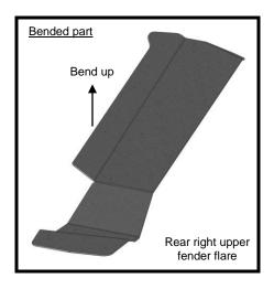
i) For this step, the help of another person is strongly recommended. The use of clamps and/or tape to hold the fender flare in position during this step may be helpful as the fender flare needs to stay in place while you drive in the self-drilling screws.
