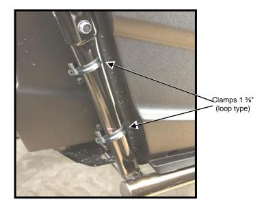
**m**) Without tightening, attach the rear right lower fender flare part to the loop clamps installed in step l) using supplied hardware (Item G) as shown.
