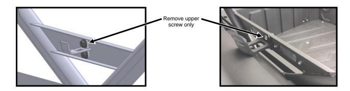
f) Install the windshield to the vehicle using supplied hardware (Item E) as shown below. Adjust the position of the windshield and tighten. <u>Caution: over tightening any hardware could cause irreversible damage to the windshield.</u>
