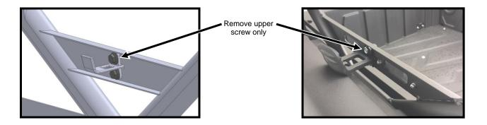
f) Install the windshield to the vehicle using supplied hardware (Item E) as shown below. Adjust the position of the windshield and tighten. Caution: over tightening any hardware could cause irreversible damage to the windshield.
