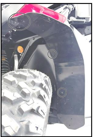
c) Ensure that the front left fender flare is properly positioned and use the remaining mounting holes (14x) as a guide to drill <sup>5</sup>/<sub>16</sub> inch diameter holes through the vehicle's front fender. For this process, drill one hole at a time and secure with push type retainer (Item H). Repeat in that order as shown below.
