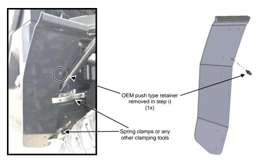
I) Use the remaining mounting holes (9x) as a guide to drill  $\frac{5}{16}$  inch diameter holes through the vehicle's rear fender. For this process, drill one hole at a time and secure with push type retainer (Item H). Repeat in that order as shown below.
