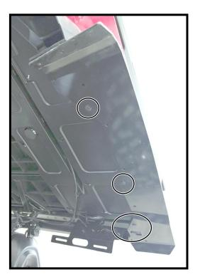
g) Use the remaining mounting holes (8x) as a guide to drill  $\frac{5}{16}$  inch diameter holes through the vehicle's rear fender. For this process, drill one hole at a time and secure with push type retainer (Item H). Repeat in that order as shown below.
