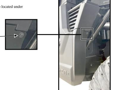
**j**) Apply the co-extruded <u>SIDE</u> bulb seal (Item G) to the rear left lower fender flare (Item E) edge as shown below using manual pressure to ensure good adhesion and cut any excess.
