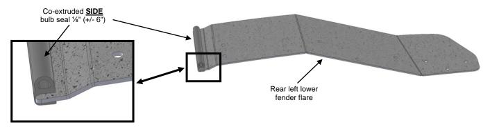
**k**) Attach the rear left lower fender flare part to the OEM fender using the OEM push type retainer removed in step i) and temporarily secure the remaining section of the rear left lower fender flare to the vehicle using spring clamps or any other clamping tools as shown below.
