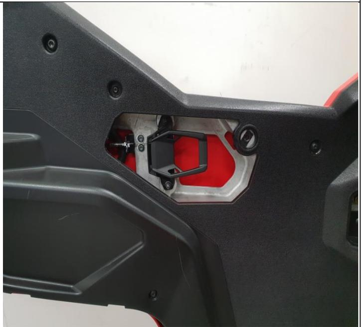
5) Remove the complete inner door panel.
