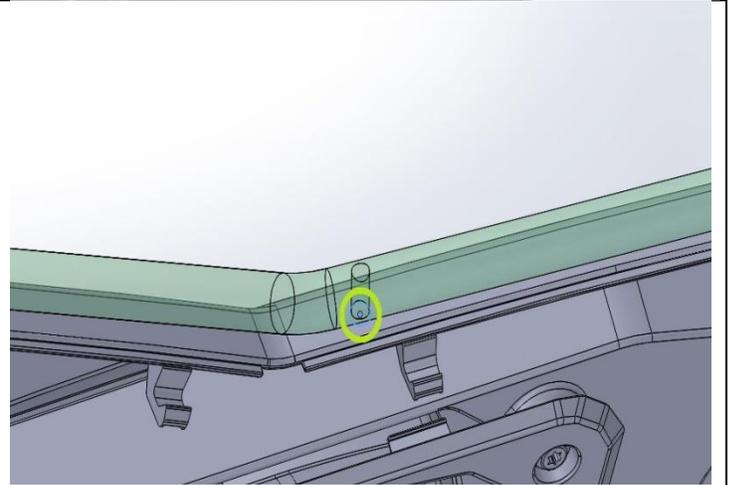
25) Remove the upper door. Install the Jack nut in the marked location.
