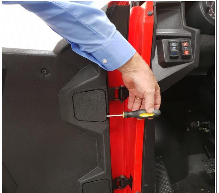
3) Remove the screws as shown. Make a note of the correct location of each screw to ensure they are reinstalled correctly.
