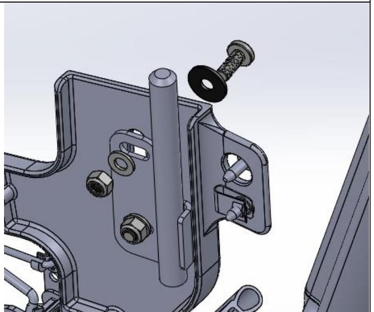
14) Remove the upper front vehicle hinge from the aluminum casting. Save the hardware for use in the next step.
