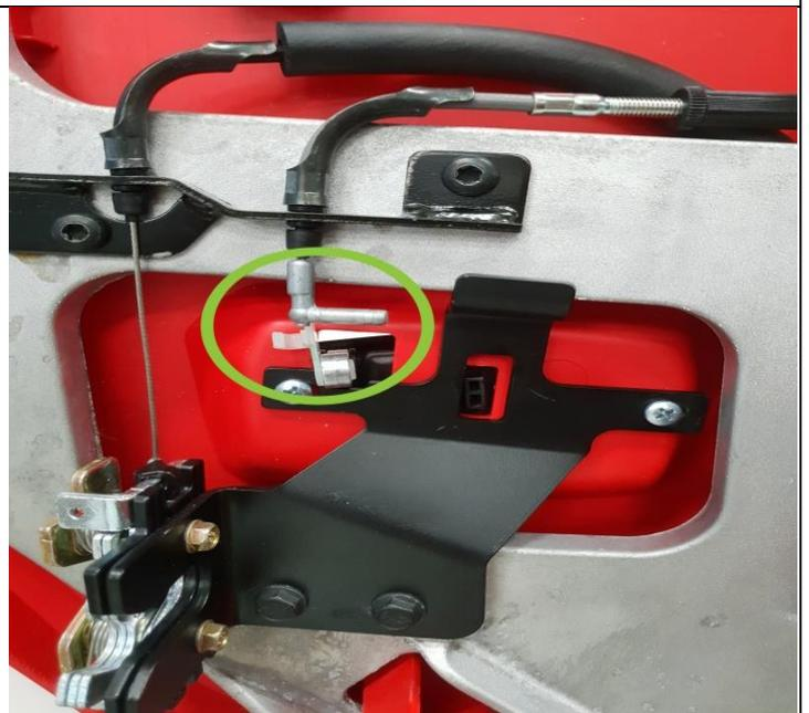
8) Remove the outer handle screws and remove the outer handle.
