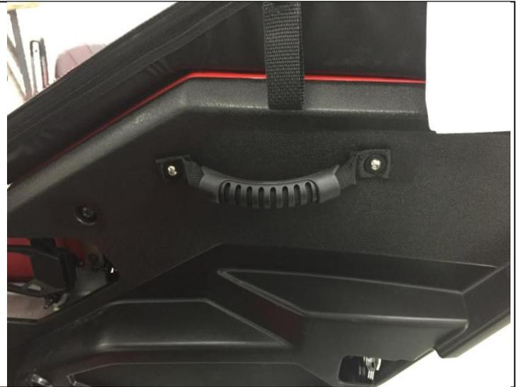
24) Reinstall the upper door and double check the fit. Close the door, and unzip the lower interior fabric (note: this is a separate zipper from the window zipper). Using an awl, mark the location for the jack nut and thumb screw through the frame and into the lower door plastic panel. Be sure to mark through the opening in the lower door and do not pierce the fabric.
