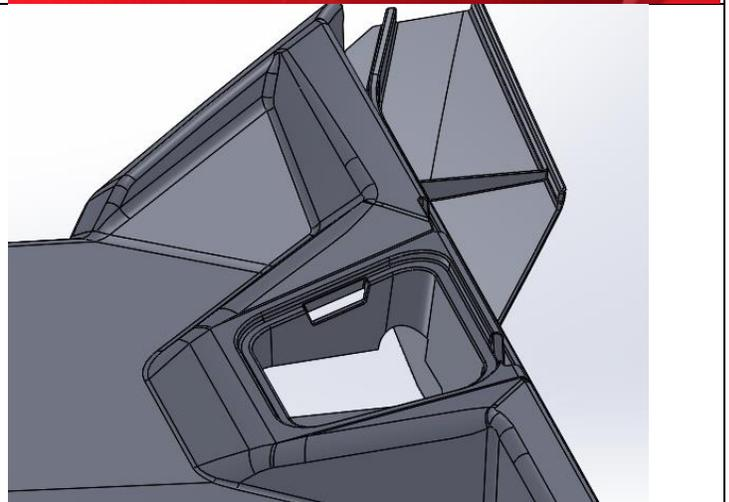
23) On the left side only: Install the interior handle by removing the rear top bolts and placing spacers in the locations and bolting down the handles using the M6x35mm bolts with washers.
