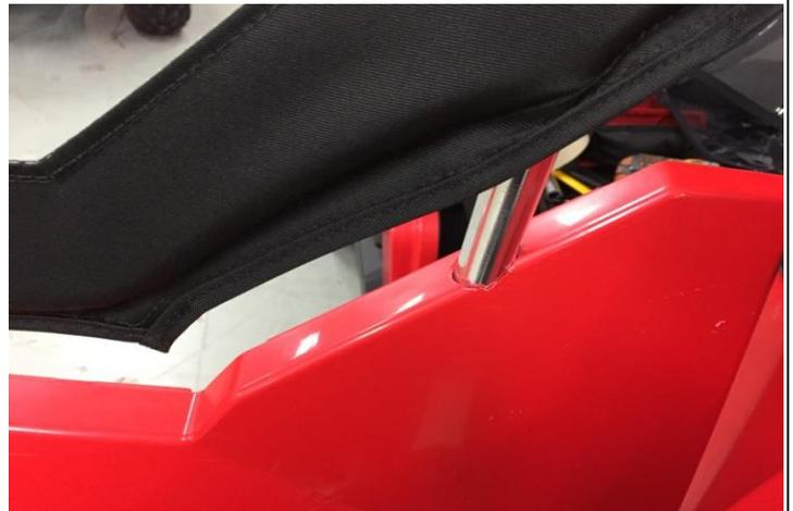
22) Reinstall all plastic panels and handles in the reverse order of removal. Be sure to reconnect all latch cables to ensure correct door operation. The upper door should be easy to install and remove through the holes cut in the previous step. Interior panels will need to be notched (Dremel and sanding bit) as shown to clear front receiving brackets.
