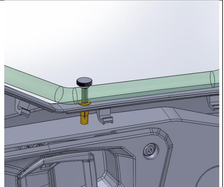
26) Reinstall the upper door. Install the thumb screw into the jack nut.
