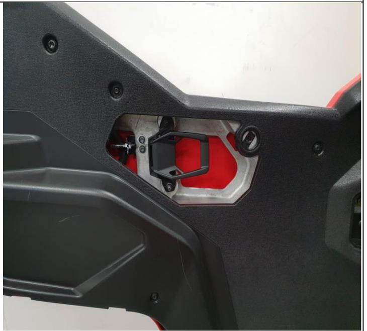
5) Remove the complete inner door panel.
