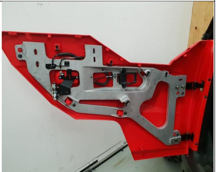
6) Remove the outer door handle-cable by pushing the plastic cable lock towards the outside of the door.
