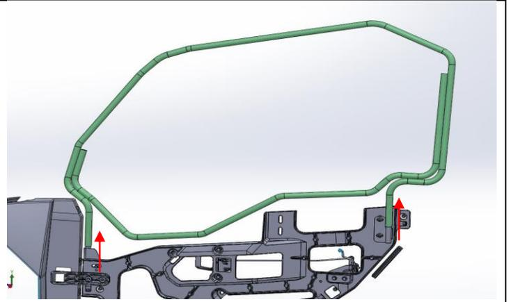
20) Place the exterior plastic panel onto the door frame in the correct location and mark the locations of the receiving brackets.
