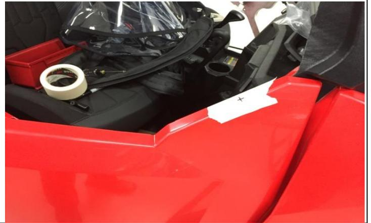
21) Trim the exterior plastic panels. Begin by drilling a small (approximately 0.125") hole in the marked locations. Visually confirm that the holes are centered above each receiving bracket pin. Gradually increase the drill size to a 0.875" diameter bit, while confirming the hole remains centered.
