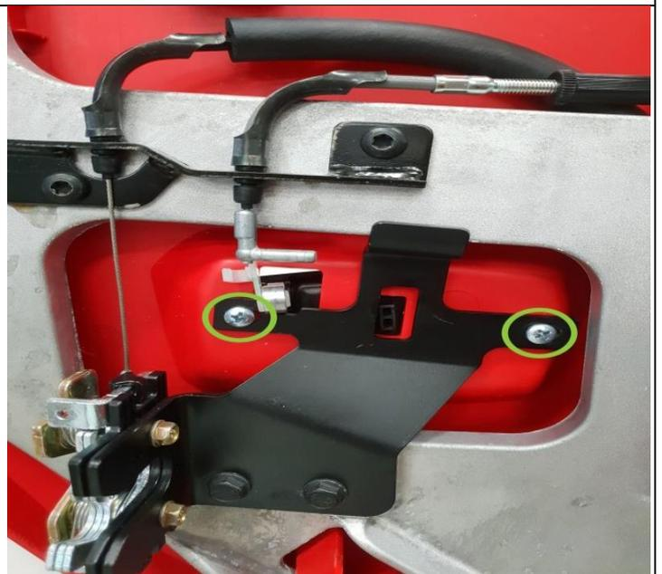
9) Remove the outer panel screws as shown.
