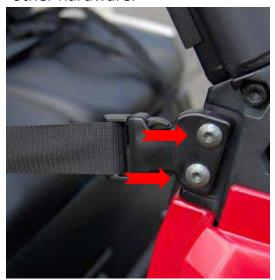
2) Remove 6mm bolt that secures net. Retain bolt with net and other hardware.
