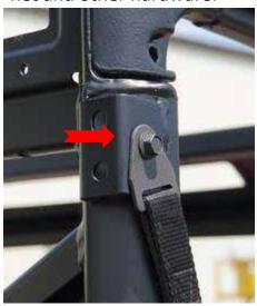
3) Using flat head screwdriver, as shown, remove rubber plug to allow removal of front lower net rod.
