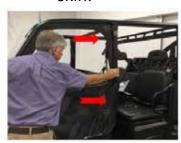
32) Close door and whole holding front of door tight to ROPS, tighten (2) 6mm rotary latch bolts.
