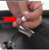
25) Insert bolt with cable up through rotary latch. Install 6mm locknut. Adjust cable so it has about ¼" slack and tighten locknut. Insert open end of cable through shrink tube. Heat shrink with heat gun or lighter.
