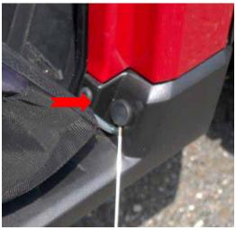
4) Remove lower T40 torx screw on unit floor (net bracket). After removing net bracket, reinstall torx screw.
