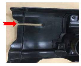
14) Install lower left-hand side hinge bracket. Center bracket on torx screws front to back and torque the (3) 8mm screws to 16 ft./lbs.
