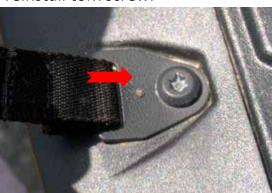
5) Remove upper (2) T40 bolster screws and set aside for use later.
