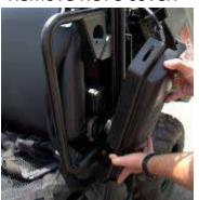
11) Remove 8mm. lower bolt for net and bolster bar.
