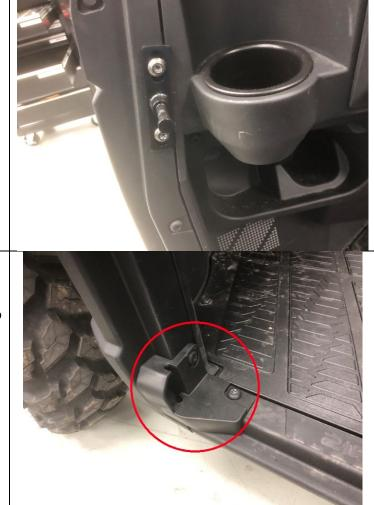
Remove all of the side net brackets. The lower rear bracket and hip restraint bracket are secured with T40 Torx screws.
