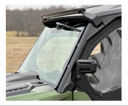
When installing the Spike Power Sports upper door kit for the Yamaha RMAX-4, the shroud clips (referenced on page 9, step #2 of the instructions) will not be used. The shroud will be held in place by the left and right support pillars which are included with the OEM glass windshield kit.
