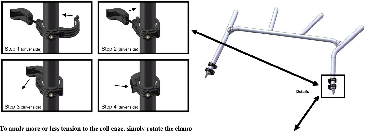
**To apply more or less tension to the roll cage, simply rotate the clamp handle from the tension screw as shown below. Over tightening clamps to roll-cage could cause parts failures.**
