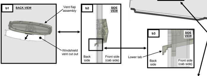
b. Install the remaining vent components (Item C) using supplied hardware as shown below in image b4 & b5.
