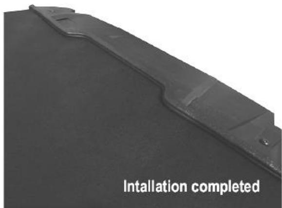
d) Install the roof (Item A) to the vehicle as shown below.
